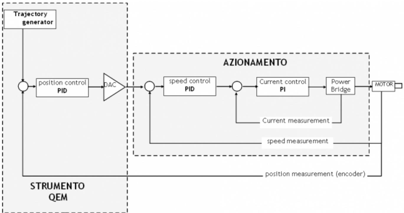
QEM instrument implements the trajectory and loop position generator.
