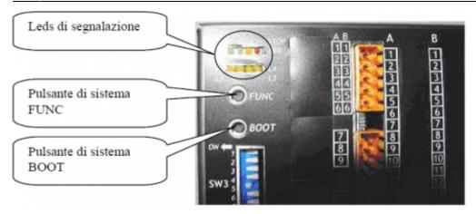
**4.**Switch the instrument with the **FUNC** button pressed.
