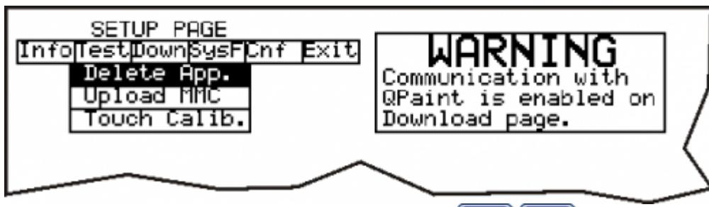
7. Select **Upload MMC** from the menu using the arrows of the virtual keyboard, then press the for show the System Functions.
