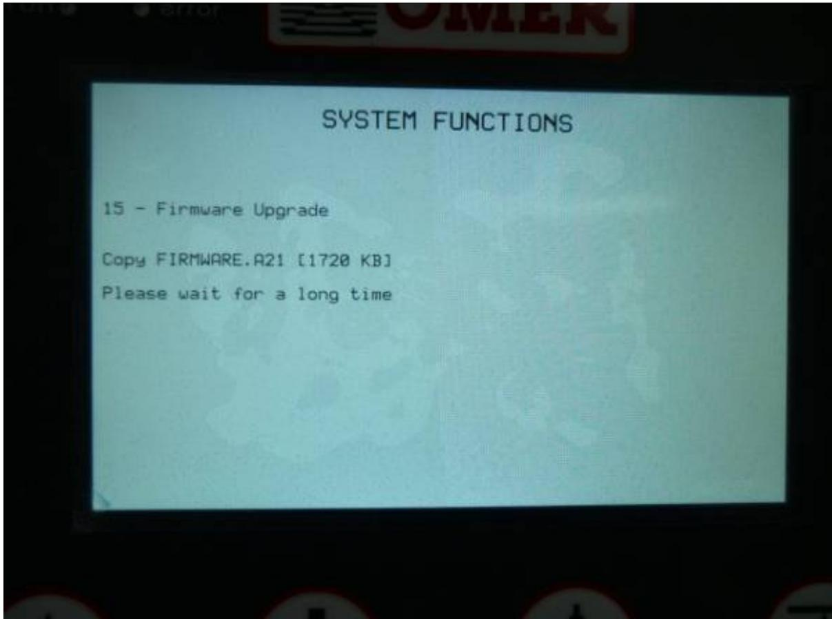
9. When you have finished, The following screen is showed for 5 seconds and then the MQ5CF automatically restarts.
