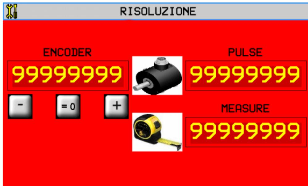
When the axis resolution cannot be calculated mathematically with the machine data, this page is a tool for the experimental calculation of resolution, or to check it.
