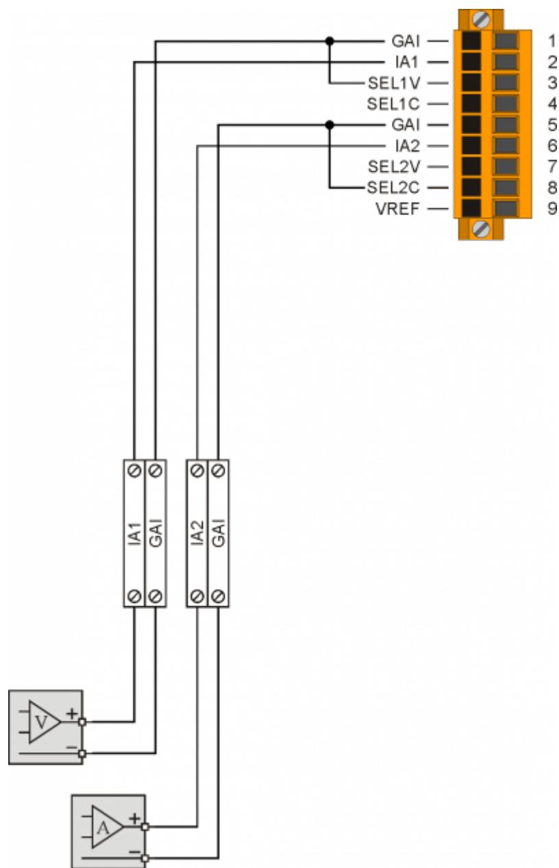
**Voltmetric and potentiometric analog inputs**
