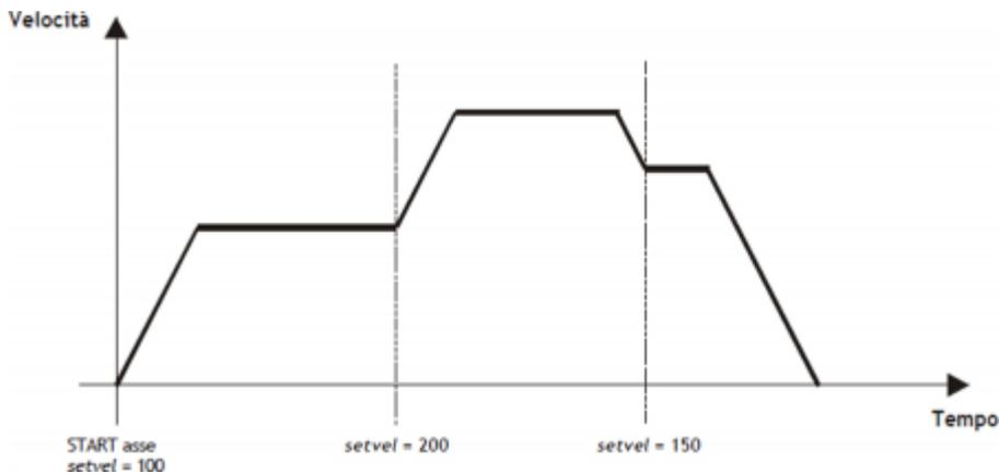
When positioning can be varied even acceleration/deceleration times. For example, the device can start a placement at a rate very short and once they reach the speed set, varied *tacc* parameter and executed a change of speed with a very long ramp. For special applications and trapezoidal ramps, ramp time can be varied even during a change of speed, in this case the new time is put into execution immediately.
