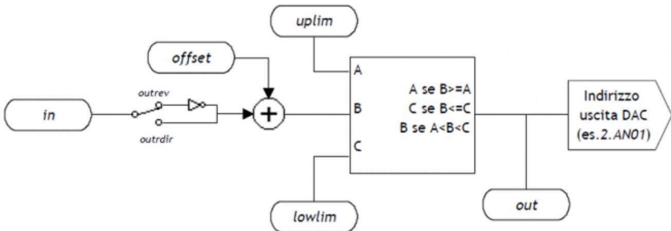
The DAC device, since it works with 16 bit resolution, accepts input values between -32768 and 32767. The output voltage is proportional to the value entered by the user. The device has a symmetrical behaviour around the zero analog voltage at less than any offset value entered. The minimum and maximum analog voltages can be set by the lowlim and uplim parameters, always remaining within  $\pm 10V$ :
