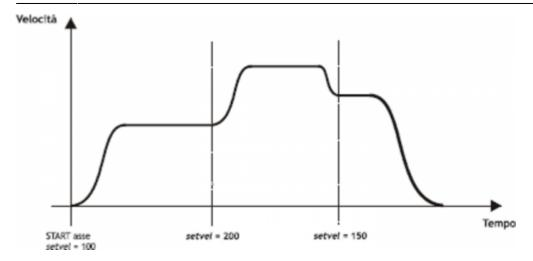
When positioning can be varied even acceleration/deceleration times. For example, the device can start a placement with a very short ramp and, reached the speed set, the *tacc* parameter is changed and executed a change of speed with a very long ramp.
