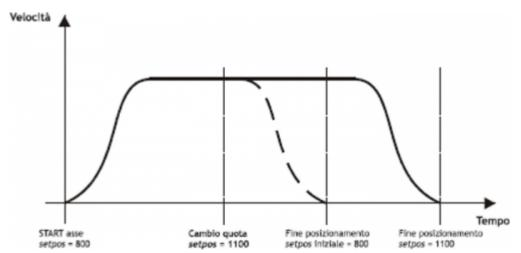
When positioning you can also change the value of the *posit* count. This function is usually used when a device must, under special conditions, continue a speed profile for a very long time, that exceeds the time axis takes to reach the limit quota (*maxpos* or *minpos*).
