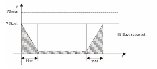
N.B.: In the graph represented the speed could become negative (and then push back the Slave) if the case of the Slave space set is lesser of the space covered for the acceleration and deceleration ramps.
