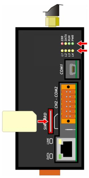
Slot for SIM card (highlighted by the arrow)
