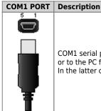
COM1 serial port TTL standard electric used for connection to a QMove+ product (DIP 8 of SW1 OFF) or to the PC for the Bridge configuration (DIP 8 of SW1 ON). In the latter case, you must use the IQ009 or IQ013 accessories.
