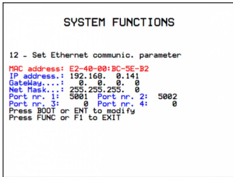
The port set in "Port nr.1:" represents a communication channel equivalent to PROG PORT. The port set in "Port nr.2:" represents a channel equivalent to USER PORT. The ports 3 e 4 are not used.
