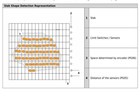
• check the functionality of the slab detection sensors on the DIAGNOSTICS 2 page. If the limit switches detect the presence of the slab, the LEDs light up.
