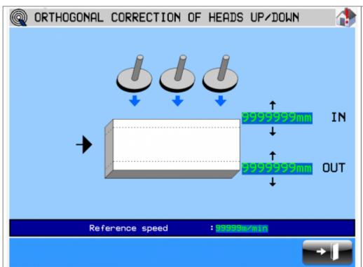
Page where you need to act to anticipate / postpone the heads. In the parameter "reference speed" you need to insert the speed of the bridge. If you dont put a value in "reference speed", the correction parameters are not adapted to each speed change of the bridge.
