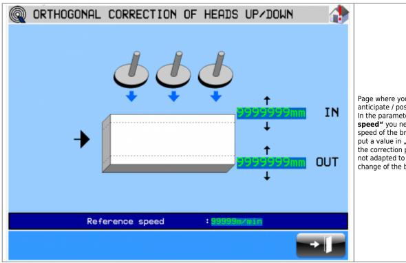
Page where you need to act to anticipate / postpone the heads. In the parameter "reference speed" you need to insert the speed of the bridge. If you dont put a value in "reference speed", the correction parameters are not adapted to each speed change of the bridge.
