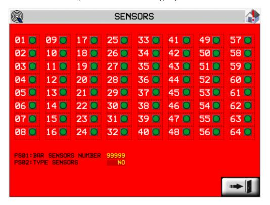
• set the parameter PG05:Orthogonal Step (distance of the sensors) and the parameter PG06:Horizontal Step (space determined by the encoder) in the generic SETUP page
