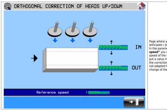
Page where you need to act to anticipate / postpone the heads. In the parameter "reference speed" you need to insert the speed of the bridge. If you dont put a value in "reference speed", the correction parameters are not adapted to each speed change of the bridge.
