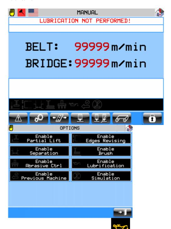
Lubrication is performed if the command on the Options page Enable Lubrication is active. This command allows you to perform lubrication cycles in time.
