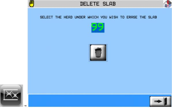
Select the head under which you want to delete the slab and press the delete button.
