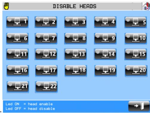
On this page, you can see the status of each head. LED on = head enabled; LED off = head disabled. Head enabling and disabling is done through the selector.
