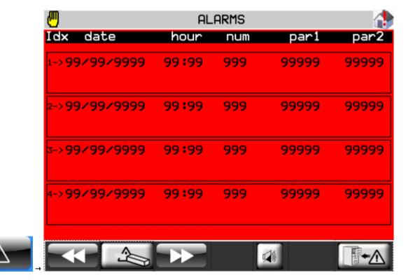
With the button, you can clear the current messages and restore the machine's operation after a few seconds of waiting. If some alarm causes are still present, the alarm messages will reappear. If there are no active alarms, the machine will automatically return to the main page after 2 seconds.
