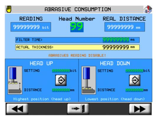
To perform operations / view data on this page, it is necessary to have the parameter PG 12 = ON and the "Enable abrasive CTRL" option active.
