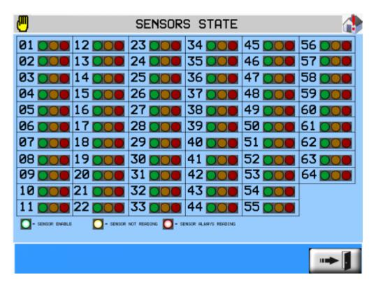
On this page, you can see the status of all sensors. Green LED = enabled sensor Yellow LED = warning, the sensor is not reading Red LED = alarm, the sensor is always reading
