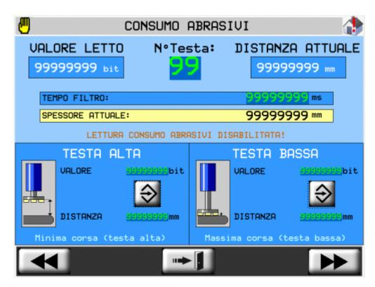
Calibrate the input for abrasive thickness reading on the "consumo abrasivi" page.
