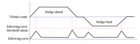
With the gantry in motion, lower the tracking error value (following error) from 9999 to 100. Gradually reduce it from 100 towards 0000. Once you find the value that triggers the alarm, add 15%. Caution: The MAX and min tracking errors must be less than 30.
