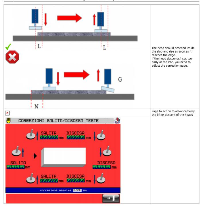
Raise the speed of the bridge and belt, then check that the lift and descent remain correct. In case they change, check the advance of lift or descent on the dedicated page and modify if necessary.
