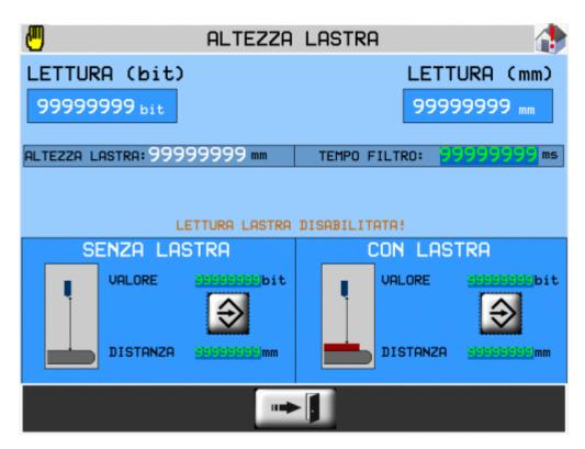
Calibrate the plate height reading input on the "altezza lastra" page.
