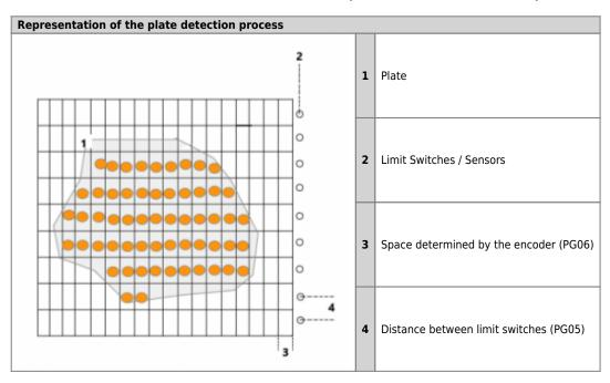
Check the functionality of the plate detection limit switches on DIAGNOSTIC 2 page. If the limit switches detect the presence of
