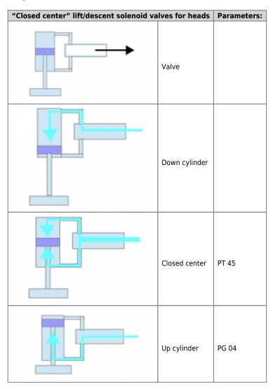
By setting the partial head lift time (parameters  $45 \div 66$ ), the lift output is de-energized after that time, and mechanically, when the lift and descent are de-energized, the upper chamber is in communication with the lower chamber of the cylinder, blocking it in that position (closed center). Full ascent will only be done when the head no longer needs to work, after the time set in parameter PG 04.
