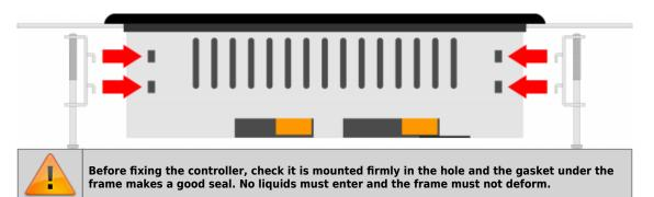
Screw the controller in place.
