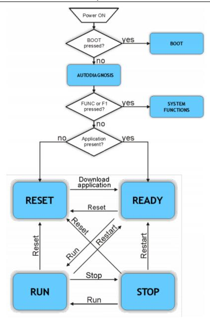
The BOOT state can be used to access the firmware updating functions.
