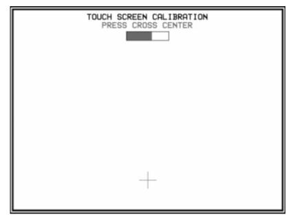
At the entrance of the procedure, it is presented with a screen where there is a blue cross. Press the center of the cross until the progress bar has reached completion.
