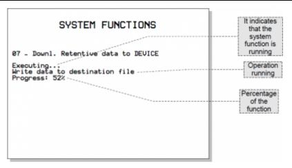
When the function ends the **POW** led stops flashing. Instruments that have a display, you see the page "SYSTEM FUNCTIONS" as in the figure below.
