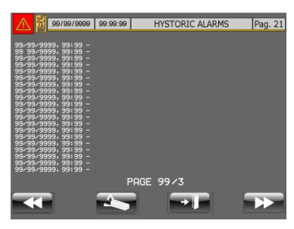
The alarm log file can contain at most 60 registrations. It is a FIFO log file, therefore when the log file is full and another alarm is registered, the oldest in the list is removed.
