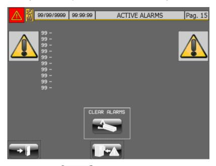
By pressing the key the alarms are cancelled. If there are no alarms, after 2 seconds the exit out of this page will occur automatically.
