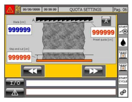
To work with the automatic speeds, it is required to set the starting value from which the device will start calculating the values of the various entries.
