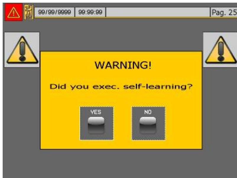
If the operator presses the key YES, he informs the device that the self-learning has been performed, therefore the device goes back to the main page.
