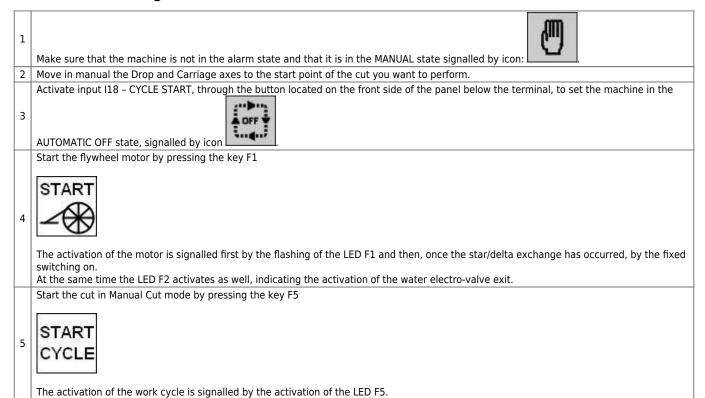
In the Manual Cut procedure the platform starts from the value where it is and goes up until value 0 (bench edge) with a speed which is regulated by the potentiometer located on the front side of the operator panel.
