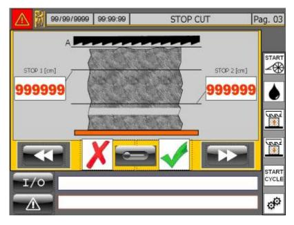
The machine is provided with the STOP CUT function: therefore you can program until 2 intermediate stops during the slab cut.
