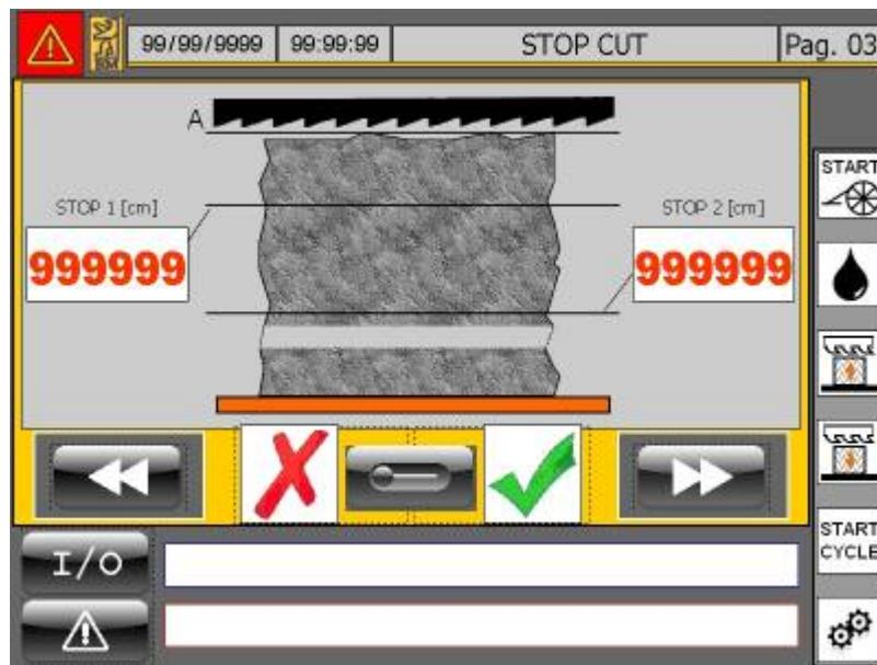
The machine is provided with the STOP CUT function: therefore you can program until 2 intermediate stops during the slab cut.
