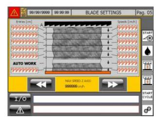
This page sets the entry speed of the blade into the material to be cut during the automatic cut.
