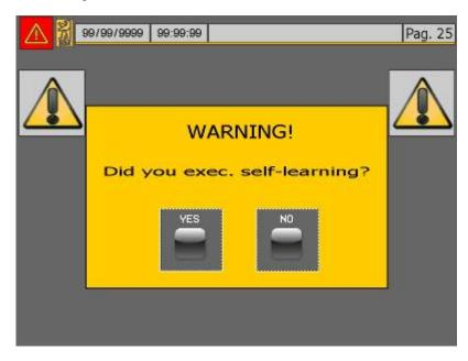
If the operator presses the key YES, he informs the device that the self-learning has been performed, therefore the device goes back to the main page.
