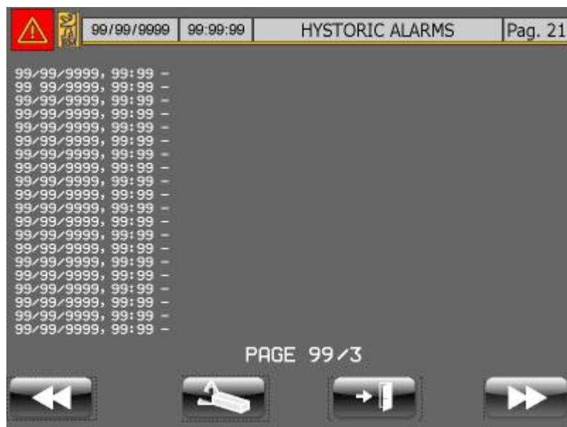
The alarm log file can contain at most 60 registrations. It is a FIFO log file, therefore when the log file is full and another alarm is registered, the oldest in the list is removed.
