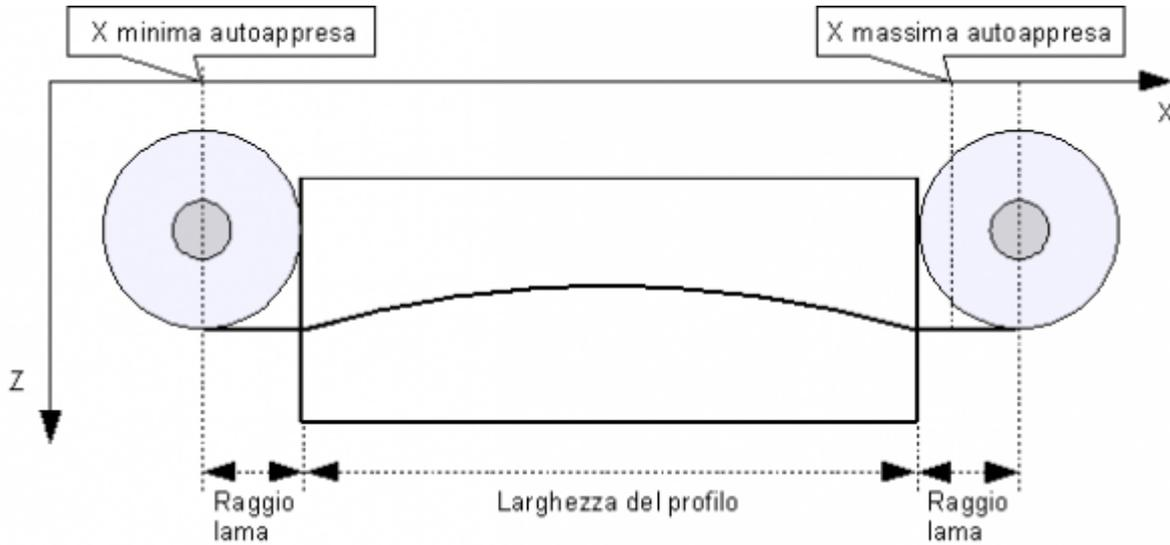
Profile width + disk diameter is greater than the two self-learned X points. As shown, the cut starts at the self-learned minimum point and is completed when it passes the self-learned maximum X point.
