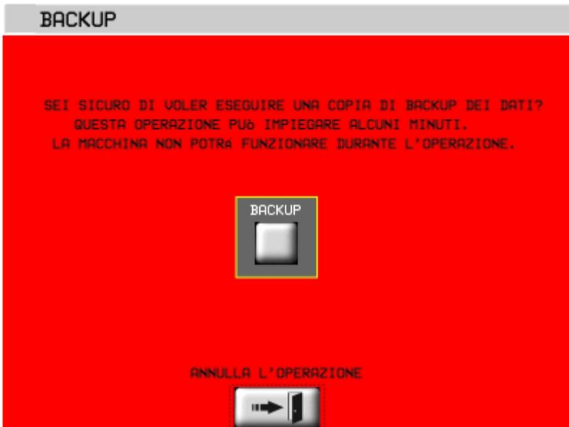
This procedure saves all machine data and parameters on the controller's internal memory.
