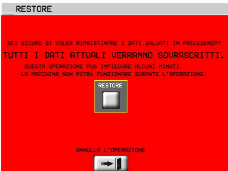
This procedure restores the machine data and parameters saved on the controller's internal memory. The Backup procedure must have been performed before using Restore.
