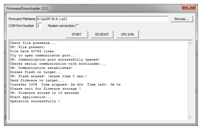
All messages, including any errors, appear in the notification area. If the procedure ends correctly, will appear the **"Operation successfully"** message and the instrument will automatically start.
