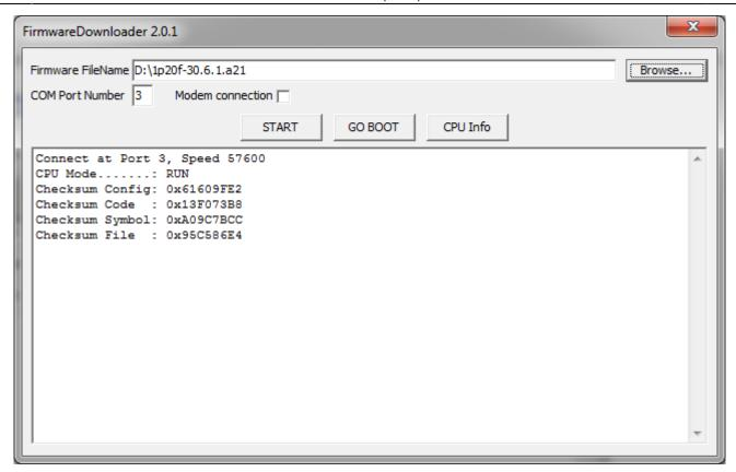
If the connection is correct, the speed data will be showed to the instrument where the port is configured, The CPU status and checksums for the QCL application.
