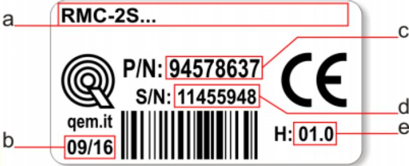
The image shows a product label for RMC-2S... with callouts: 'a' points to the model number 'RMC-2S...'; 'b' points to the production date '09/16'; 'c' points to the part number 'P/N: 94578637'; 'd' points to the serial number 'S/N: 11455948'; 'e' points to the hardware release 'H: 01.0'. The label also features a QR code, a barcode, the website 'qem.it', and a CE mark.
