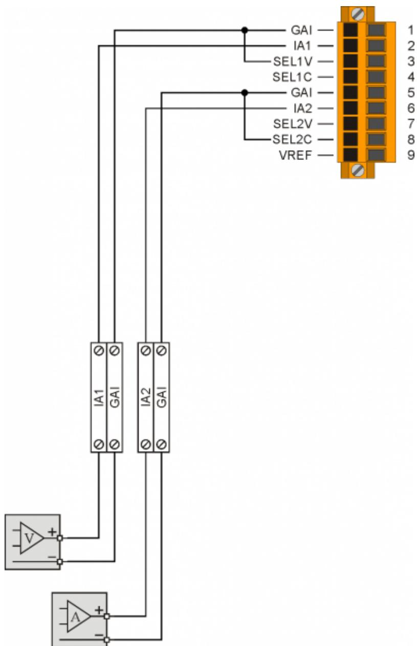
**Ingressi analogici voltmetrici e potenziometrici**
