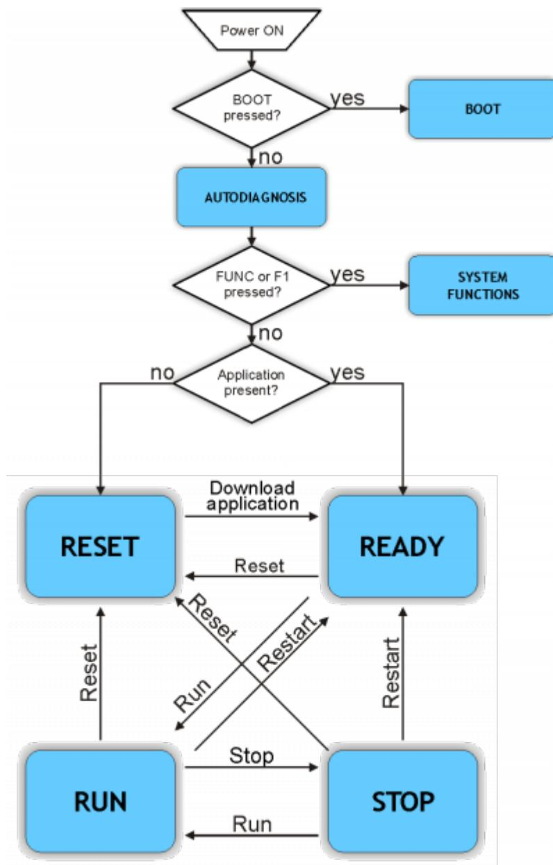
The BOOT state can be used to access the firmware updating functions.
